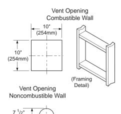
Figure 22 - Vent Opening Requirements
